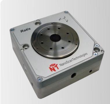
**Ratis** is a family of plane-parallel piezo stages for nanopositioning and scanning developed by NST. Piezo stages are made of solid metal bar processed with EDM wire-cutting and precise CNC machining. Movable central part hangs on flexible springs and is driven with piezo actuators. Ratis design provides excellent linearity and flatness of the
